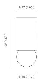
Bulb specifications 120V / 240V G9 3,5W LED Bulb 350Im / 2700K
