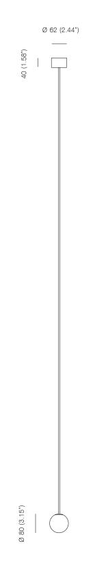
Bulb specifications 120V / 240V G9, 25W frosted halogen bulb 260Im / 3000K
