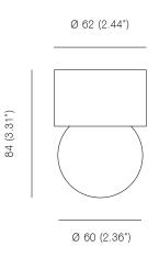
Bulb specifications 120V / 240V G9, 25W frosted halogen bulb 260Im / 3000K
