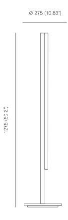
Bulb specifications 120V / 240V S14s opal LED tube Radium Raledina 16,5W / 1000mm Ø 29mm 1000lm / 2700K
