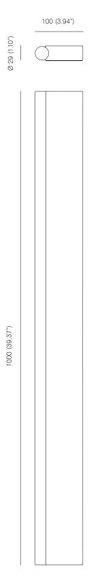
Bulb specifications 120V / 240V S14s opal LED tube Radium Raledina 16,5W / 1000mm ø29mm 1000lm / 2700K
