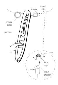
Loosen the lock cap and push the valve on the cable gripper and adjust the position of the cable gripper so that the aircraft cable is roughly the same length as the coaxial cable.
