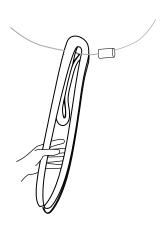
1 Lift glass off of lamp holder assembly and hold securely.
