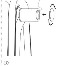
Screw frame cap back onto the frame assembly.
