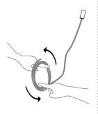
Very carefully uncoil the braided coaxial cable in a spool like manner. Insert your index fingers into opposite sides of the roll then rotate your fingers around each other to unroll the coaxial cable.
